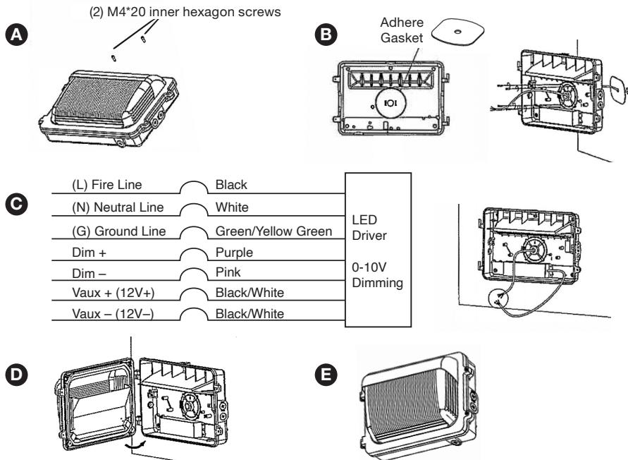
**STEP 2:** Separate the cover from the base of the fixture.
