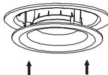
Push the LED retrofit trim into the recessed light fixture. Continue to push the LED trim until its outer edge is flush with the ceiling surface.
