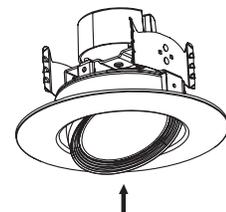
Press up one side until the other side shifts out then twist it at the desired angle. **Turn ON power.**
