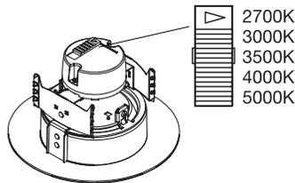
Before installation, select your preferred CCT by moving the switch to either 2700K, 3000K, 3500K, 4000K or 5000K.
