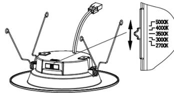
Before installation, select your preferred CCT by moving the switch to either 2700K, 3000K, 3500K, 4000K or 5000K.
