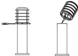
2. Forward the light cover, facing the light socket, loosen the screw, and remove the lamp.
