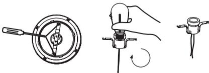
3. Screw lamps in the socket, fix the light socket to the light cover again.
