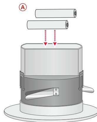
STEP 4: Re-install battery cover and BBU back in to the recessed can/housing.
