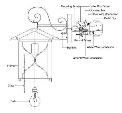
STEP 5: Use the wire connection to connect the positive and neutral wires. Connect the Ground wire to the junction box ground port.
