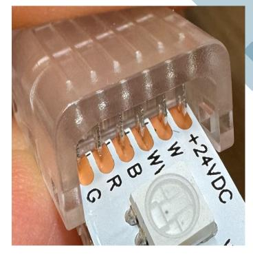
Make sure the connector is lined so the connector pins press down into the copper indicators on both ends.
