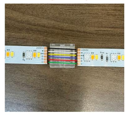
Prior to installation, make sure the tape is cut at the copper indicators. The markings of the tape must match up.
