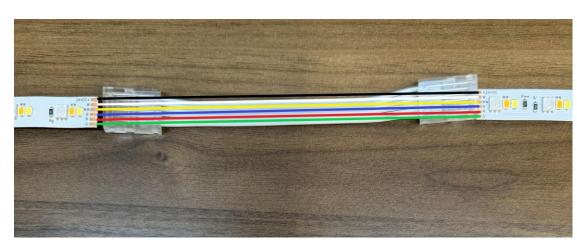
24VDC+ should line up with 24VDC+. W should line up with W. And so forth.
