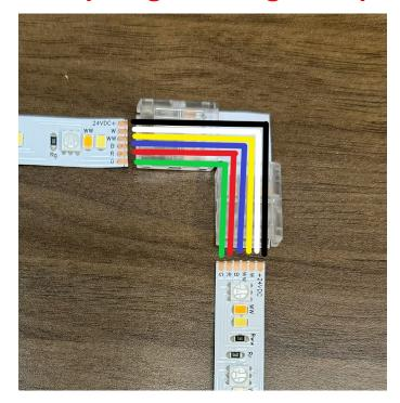
24VDC+ should line up to 24VDC+. W should line up to W. And so forth.
