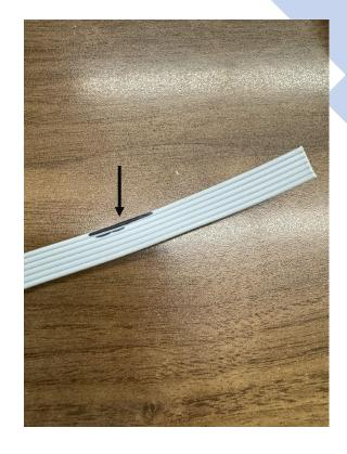
Run down to the end of the wire and indicate with black marker the wire that is connected to the 24VDC+.
