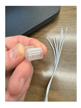
Start inserting the wires into the holes of the connector, keep the wires in the same order, do not tangle. Do not need to strip the wires.
