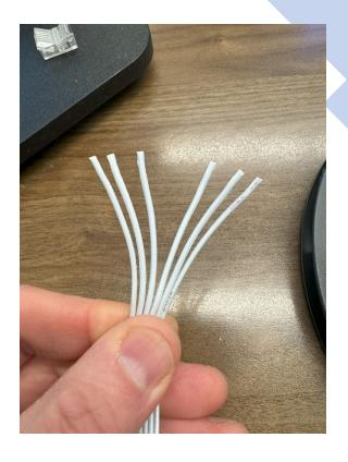
Slightly cut to get you started inbetween each wire and then pull apart to give some slack when installing into the connectors.
