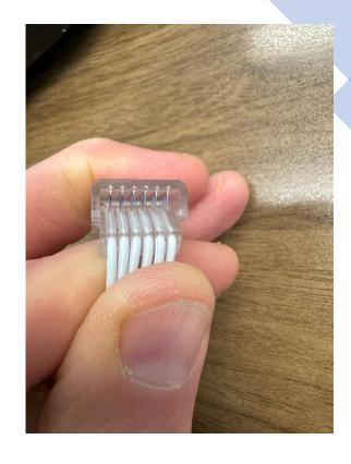
The pins will push into the wire making contact with the copper inside.
