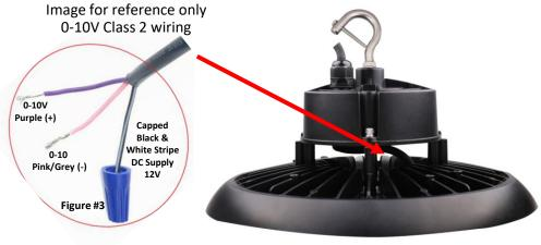
The UFO led high bay light fixture can be equipped with an optional DC motion sensor (86/218) the sensor needs to be set via remote (86/219). For Standard 0-10V dimming application, the dimming cable must be cut free from the integrated DC sensor port, see figure #2
