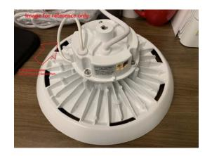
The LED high bay light can be equipped with an optional DC motion sensor (86/218). The sensor needs to be set via remote (86/219). For standard 0-10V dimming applications, the dimming cable must be cut free from the integrated DC sensor port.
