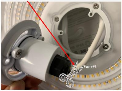
The UFO led high bay light fixture can be equipped with an optional DC motion sensor (86/218) the sensor needs to be set via remote (86/219). For Standard 0-10V dimming application, the dimming cable must be cut free from the integrated DC sensor port, see figure #2
