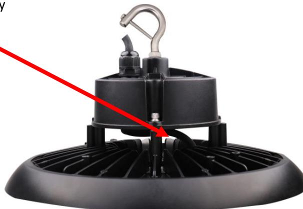
Step 2: For Standard 0-10V dimming applications, the dimming cable must be cut free from the integrated DC port to access the 0-10V dimming wires, Purple (+), Pink (-), Black with White Stripe (DC Power Supply) must be capped when using standard 0-10V controls, See Figure #3
