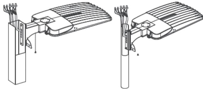
**STEP 5B:** Pass the pole wires into the fixed arm bracket, pull them out together with fixture's AC wire from junction box. Connect the fixture's AC input wires to pole wires with connectors. L to L (Black), N to N (White), PE to PE (Green). Go to STEP 6B.
