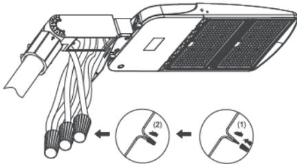
**STEP 4:** Tuck wires into junction box. Lock the cover back to junction box.
