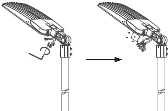
**STEP 6:** Install the cover back to junction box, tighten the screw with a wrench.
