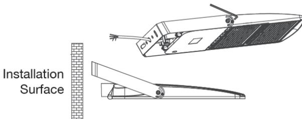
**STEP 2:** Mark the installing hole locations on the wall with yoke bracket, then drill the holes 10mm diameter with an electric drill.
