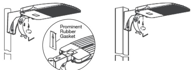
**NOTE:** When installing to a round pole, remove the prominent rubber gasket. Keep the flat rubber gasket.
