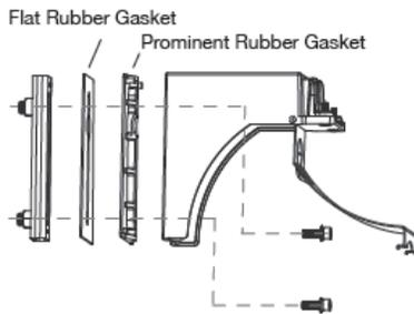
**STEP 3:** Pass the fixture's AC input wires through the fixed adapter arm bracket.
