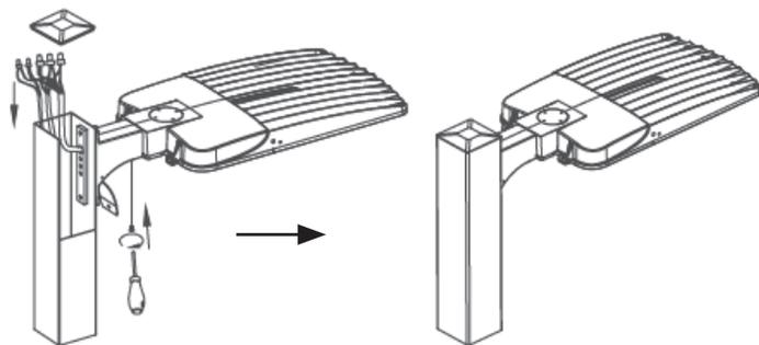
**STEP 6B:** Push the connected wires into bracket junction box, close the box cover by tightening the fixing screws, then close the poles top cover.
