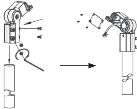
**STEP 3:** Pass the fixture's wires through the slip-fitter bracket into junction box.
