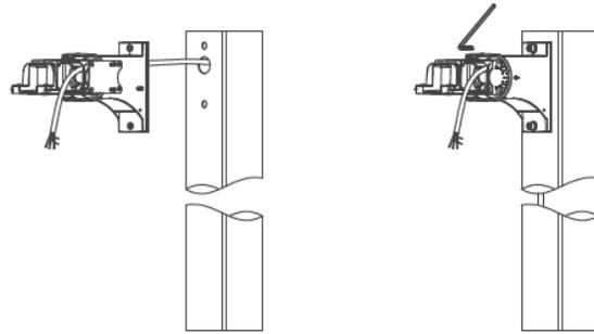
**STEP 3:** Pass the fixture's wires through the adjustable arm bracket into junction box.
