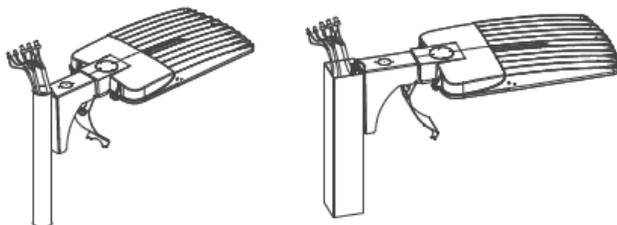
**STEP 2:** Put the iron bar inside of pole, fix it with a screw, but reserve a gap of 32mm, pass the fixed adapter arm bracket through the screw and tighten. Pass the second screw through the hole of fixed adapter arm bracket, pole and iron bar, then tighten with a wrench.
