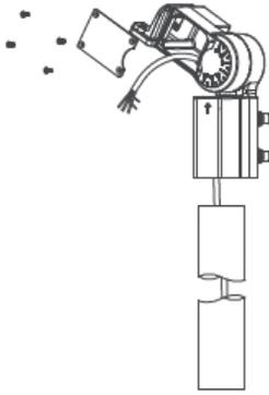
**STEP 2:** Assemble the slip-fitter bracket on the pole, tighten the fixing screws to lock with a wrench.
