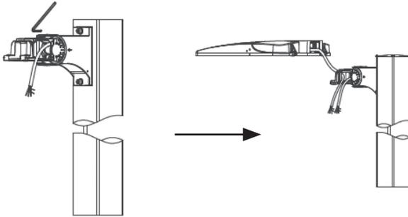
**STEP 4:** Hang the fixture body on the adjustable arm, then tighten the fixing screws to lock the fixture body with a wrench.
