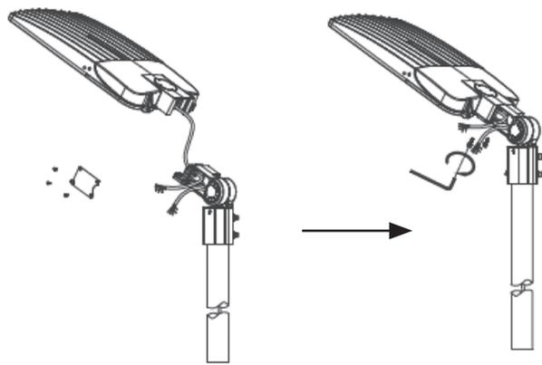
**STEP 5:** Connect the wires from pole to fixture's AC input wires, L to L (Black-Black), N to N (White-White), PE to PE (Green-Green); Connect dimming wires if desired. Use connectors to connect [Dim + ] to fixture's [Dim + ] (Purple), [Dim - ] to fixture's [Dim - ] (Pink), then put all the wire inside of junction box.
