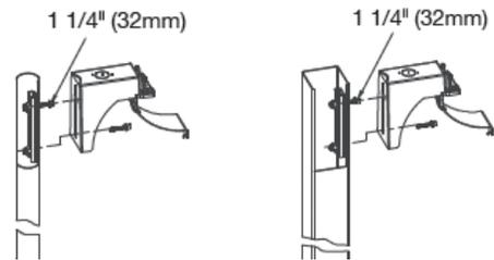
**STEP 4:** Hang the fixture on fixed adapter arm bracket. Lock the fixture by tightening screws through bracket with an allen wrench.
