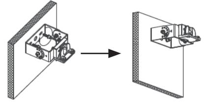
**STEP 4:** Pass the fixture's AC input wires through the trunnion bracket; then hang the fixture into the trunnion bracket, tighten fixing screws to lock it to trunnion bracket with a wrench.
