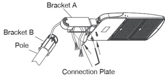
**STEP 3:** Assemble bracket A and bracket B together and fix with screw; adjust the angle needed and tighten screw. Connect fixture's AC input wires with connectors. L to L (Black), N to N (White), PE to PE (Green).
