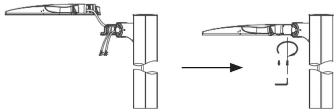
**STEP 5:** Connect the wires from pole to fixture's AC input wires, L to L (Black-Black), N to N (White-White), PE to PE (Green-Green); Connect dimming wires if desired. Use connectors to connect [Dim + ] to fixture's [Dim + ] (Purple), [Dim - ] to fixture's [Dim - ] (Pink), then put all the wire inside of junction box.
