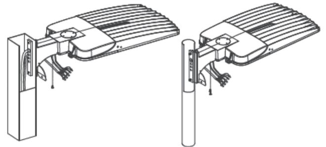
**STEP 6A:** Push the connected wires inside of the pole, close the pole's top cover, then close the junction box cover by tightening the fixing screws.
