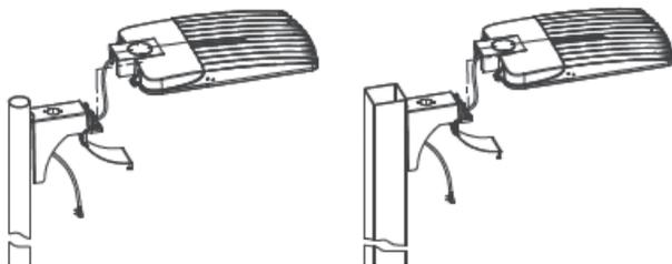
**STEP 5A:** Pass the fixture's AC input wires through the pole, pull them out together at top of pole and prepare wire connections. Go to STEP 6A on page 9.
