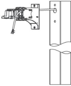
**STEP 2:** Assemble the adjustable arm bracket on the pole, tighten the fixing screws to lock with a wrench.
