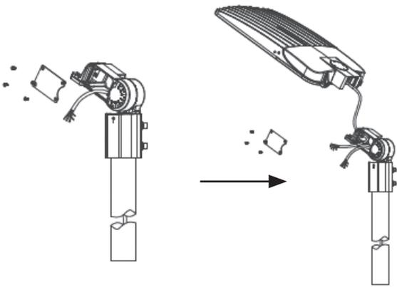
**STEP 4:** Hang the fixture body on the slip-fitter bracket, then tighten the fixing screws to lock the fixture body with a wrench.
