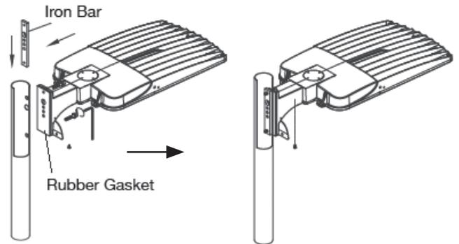
**NOTE:** When installing to a round pole, remove the rubber gasket.
