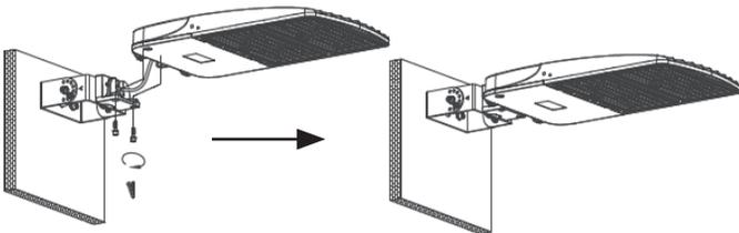
**STEP 5:** Loosen the angle adjustable screws on both sides of trunnion bracket, rotate fixture to an appropriate angle required and tighten the two screws.
