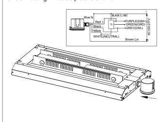
6. Again, checking the junction box and sensor are secured with screws, then completed.
