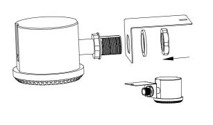
3. Loose the screws and open the junction box, then remove the knock hole.
