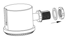
2. Installing the mounting kit on the sensor, and securing with nut.
