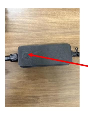
Locate and hold the on/off button on the controller for 5 to 10 seconds until all the bulbs on the string light start flashing red. String is ready to be paired to the Starfish App.
