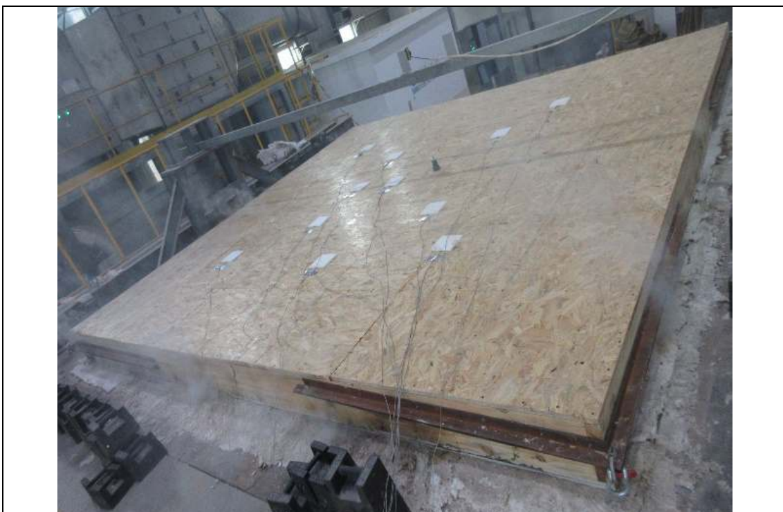
The unexposed face after test duration of 60 minutes
