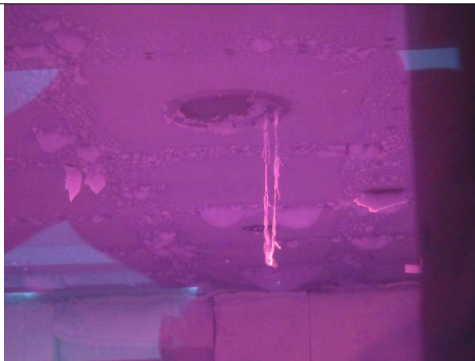
The exposed face after test duration of 15 minutes
