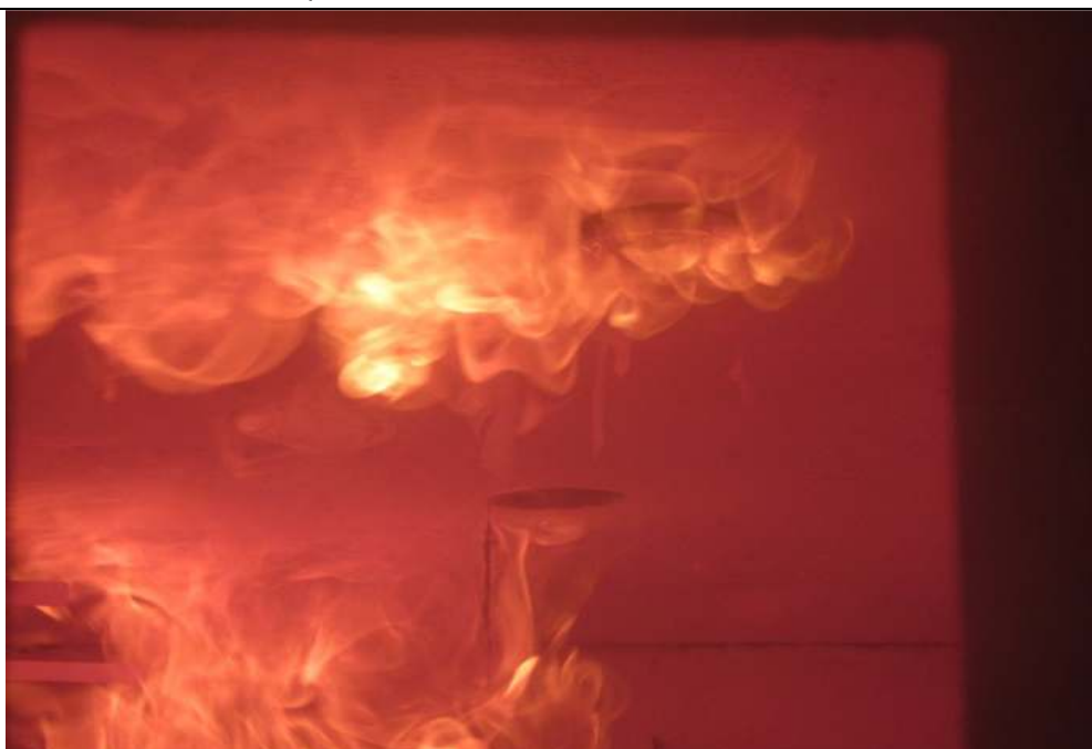
The exposed face after test duration of 120 minutes
