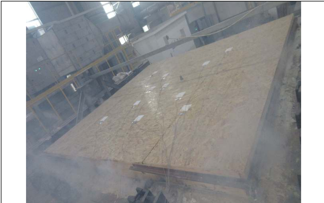
The unexposed face after test duration of 120 minutes
