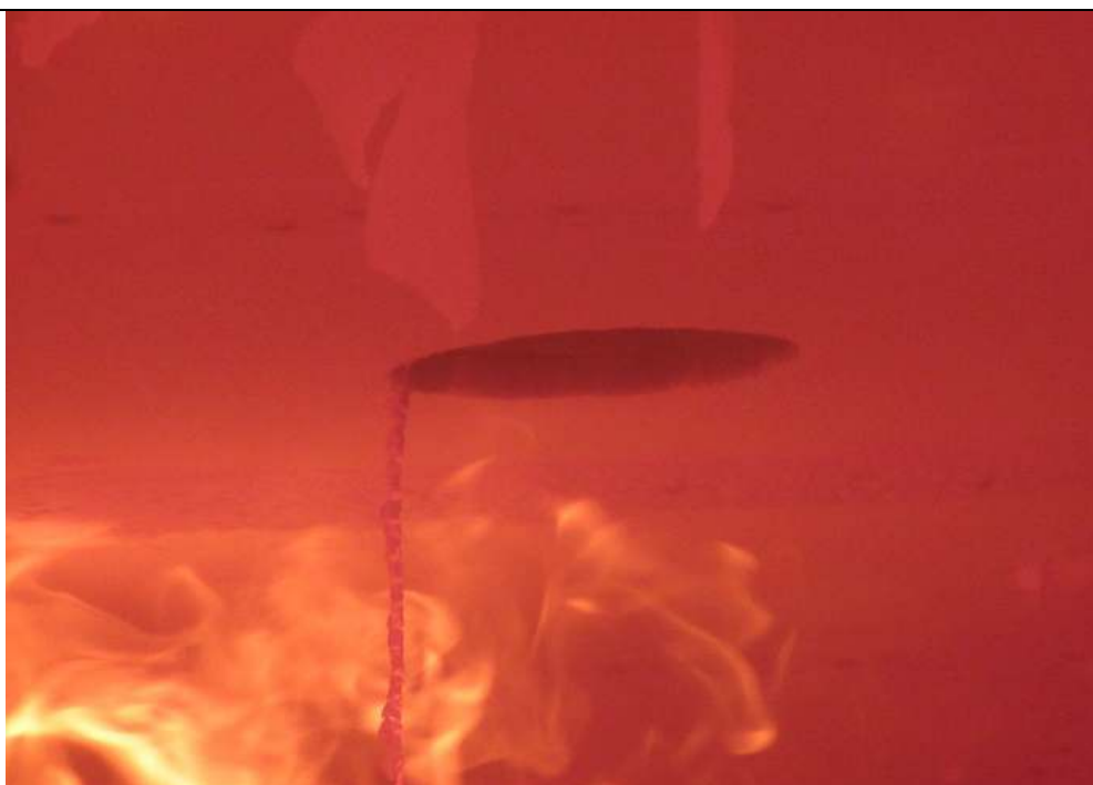
The exposed face after test duration of 110 minutes
