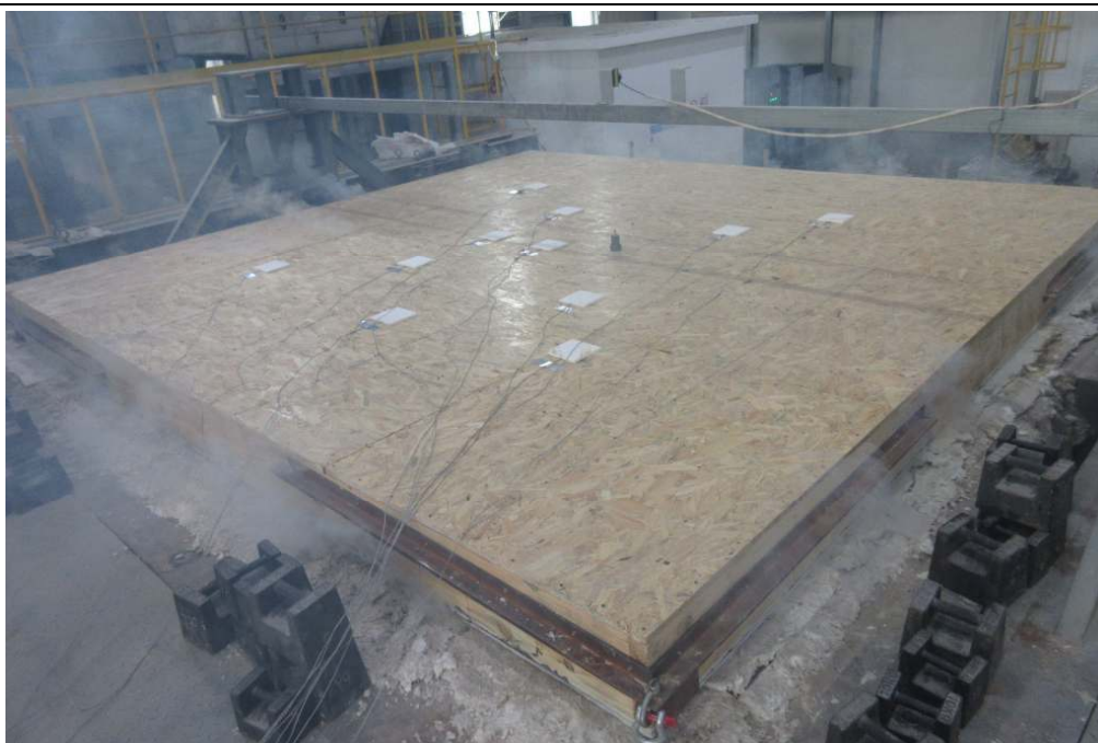
The unexposed face after test duration of 30 minutes
