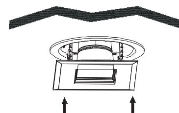
Push the LED retrofit trim into the recessed light fixture,
