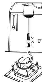
Connect the quick disconnect between the retrofit kit and the medium base umbilical socket.
