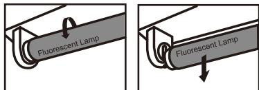
4) Bring LED lamp to luminaire and insert lamp pins into luminaire lamp holders
