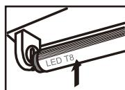
5) Rotate LED lamp until lamp locks in place. Ensure that the LED lamp front points away from the back of the luminaire.
