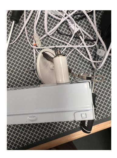
Attach the plunger into the backside of the fixture, and screw in the screw.
